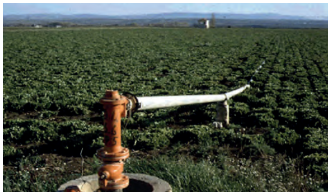
Manually controlled irrigation hydrants for opening and closing water flow in the Apulia region, Italy
