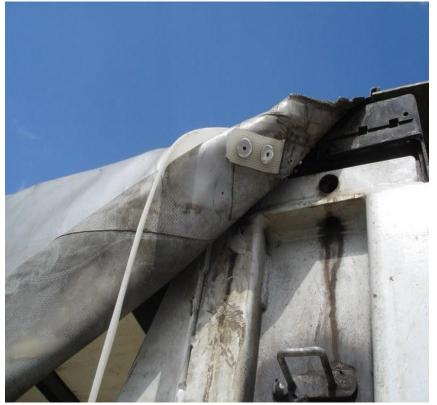
Fastening rivets of a vertical strap which cannot be replaced nor mounted to a cargo space closed with a custom seal.
