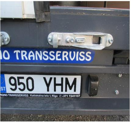
Fastening bolts of the base for the fixing handle to be fastened with nuts. A base for the fixing handle fastened to the frame with a plate with internal thread.
