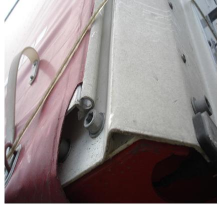
A tensioning bar without a cover flap for the curtain of the front corner for a trailer with side boards. A tensioning bar for the front corner without a curtain tensioner fixed with a cover flap and a wire cable.
