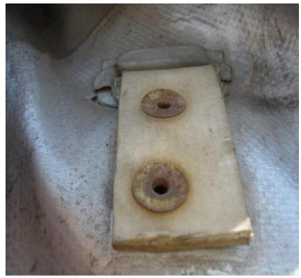
Fastening rivets of a vertical strap that can be easily mounted and replaced with hand pliers. The use of these rivets allows access to the sealed cargo space without doing any external damage or leaving external traces of the activity.
