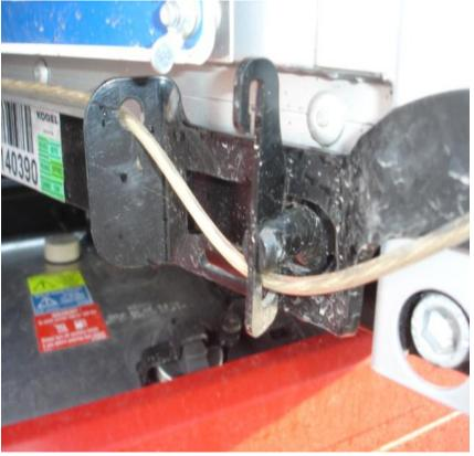
Tensioning device of the vertical rod for the side curtain to be fixed with a wire cable. A retainer for fastening the bolts of the tensioning device onto the frame.
