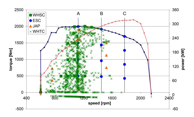
High portion of low speed operation observed, which is not representative of real world driving
