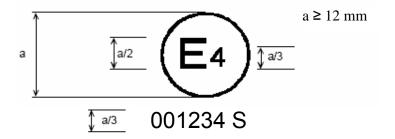
The above approval mark, affixed to a pneumatic tyre shows that a tyre concerned has been approved in the Netherlands (E4) pursuant to Regulation No. 117 (marked by S (rolling sound) only), under approval number 001234. The first two digits of the approval number (00) indicate that the approval was granted according to the requirements of this Regulation in its original form.
