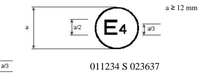
The above approval mark shows that the tyre concerned has been approved in the Netherlands (E4) pursuant to Regulation No. 117 (marked by S (rolling sound), under approval number 011234 and Regulation 30 under approval number 023637. The first two digits of the approval number (01) indicate that the approval was granted according to the 01 series of amendments, but Regulation No. 30 included the 02 series of amendments.
