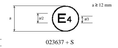
The above approval mark shows that the tyre concerned has been initially approved in the Netherlands (E4) pursuant to Regulation No. 30 and the 02 series of amendments under approval number 023637. It is also marked by + S (rolling sound) which indicates that its approval is extended under Regulation No. 117. The first two digits of the approval number (02) indicate that the approval was granted according to Regulation No. 30 which included the 02 series of
