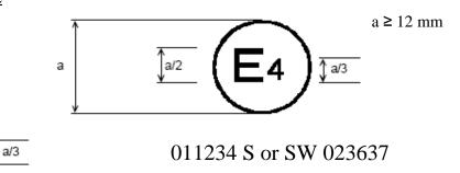
The above approval mark shows that the tyre concerned has been approved in the Netherlands (E4) pursuant to Regulation No. 117 (marked by S (rolling sound) or SW (rolling sound and wet adhesion), under approval number 011234 and Regulation 30 under approval number 023637. The first two digits of the approval number (01) indicate that the approval was granted according to the 01 series of amendments, but Regulation No. 30 included the 02 series of amendments.
