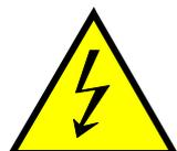
Figure 1 — Marking of high voltage equipment
