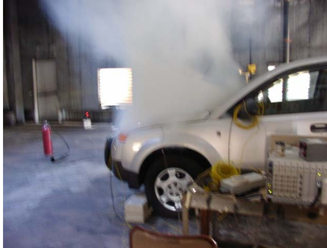
Figure 3: Fuel Line Leakage with Hood Closed
