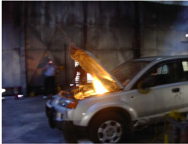
Figure 2: Fuel Line Leakage with Hood Open
