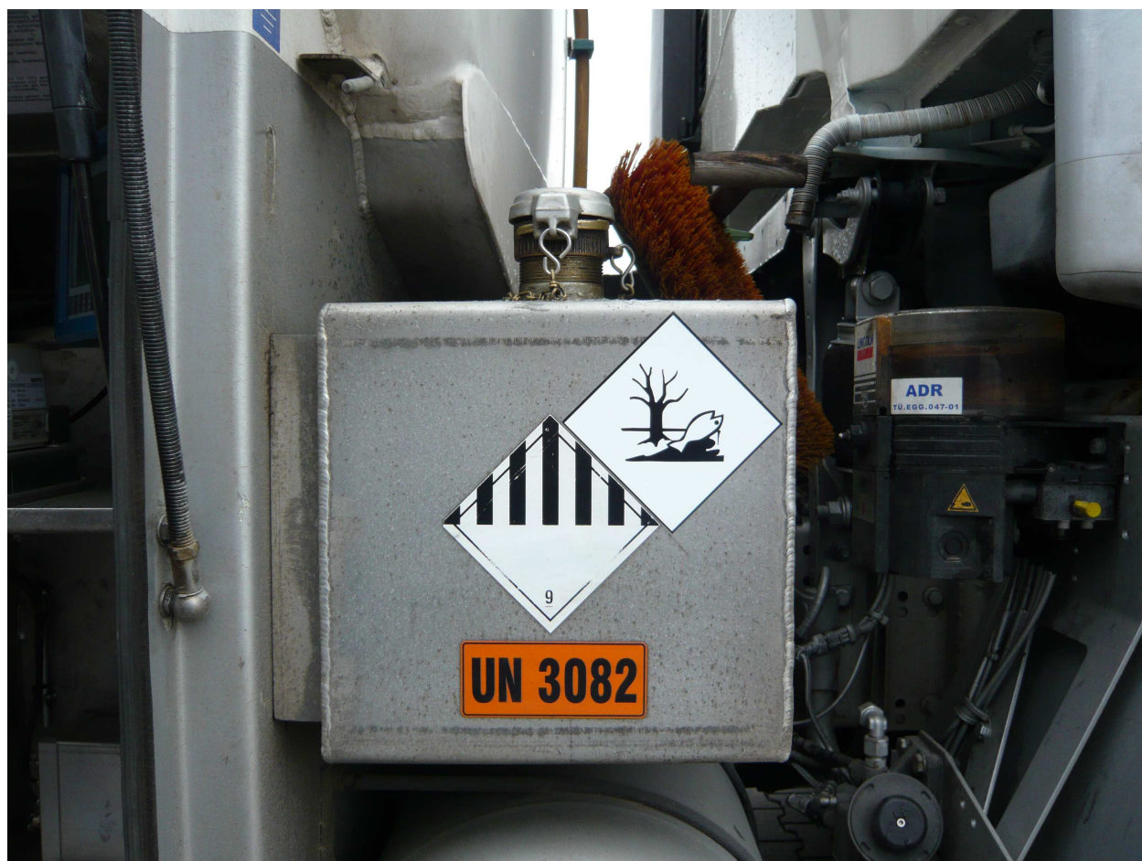
Illustration: modern additive system in the delivery system of a heating oil tank-vehicle
