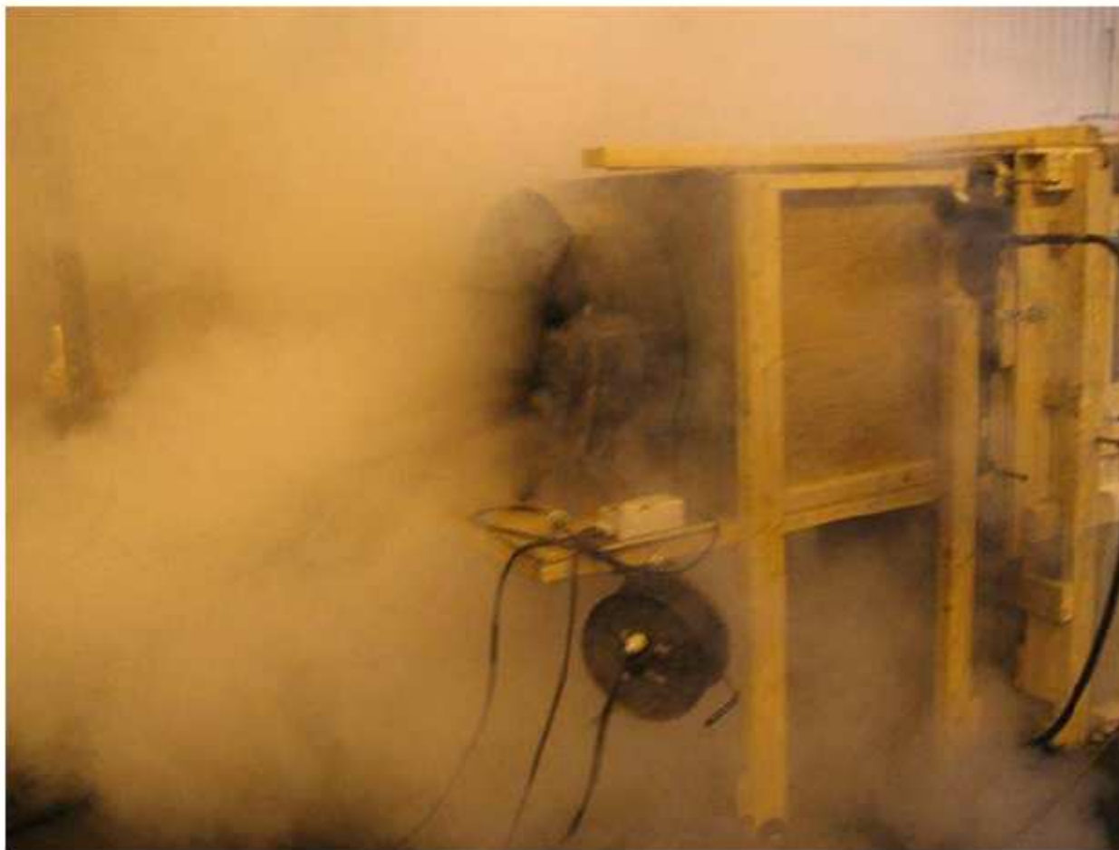
Figure 27. The extinguishing system is activated.
