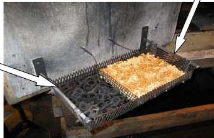
Figure 13. The smouldering rubber fire load in the net basket compartment No 1.
