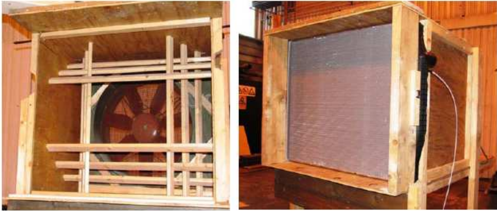
Figure 8. The axial fan with guide rails in the space. Right picture with the flow resistance
