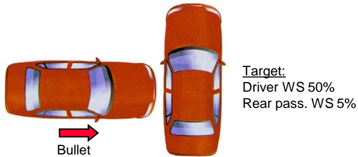
Car-to-Car & SUV-to-Car WorldSID 5% & 50%-ile
