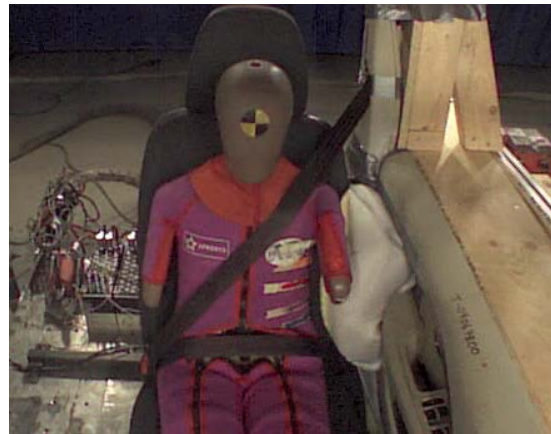
High severity MDB WorldSID 5% & 50%-ile
