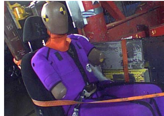
Sled test – EuroNCAP pole WorldSID 50%-ile
