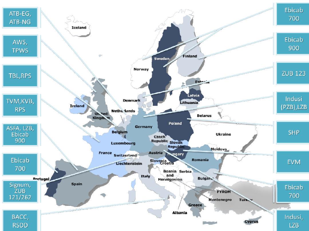
Figure 7 National train control systems in Europe
