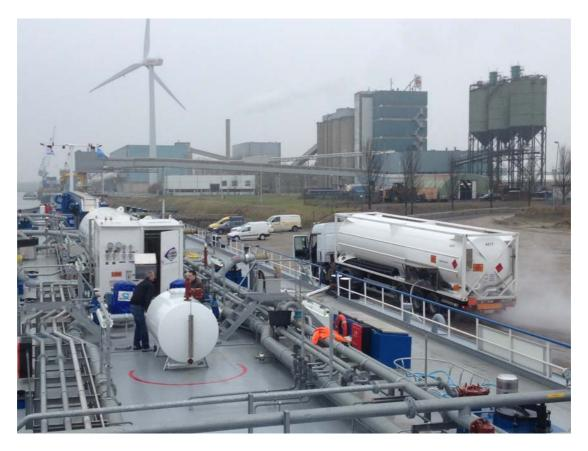
The barge sails on a mixture of 81 % LNG and 19 % gas oil (EN590). This mixture has been optimised for using the maximum percentage of LNG without decreasing the engine characteristics. The engines are Caterpillar DF3512 engines which haven't been changed for the use of natural gas. The natural gas is mixed with the combustion air before injection in the engine. During the first few weeks of the barge sailing this mixture has been changed from a 60-40 % to the final 81-19 %.
