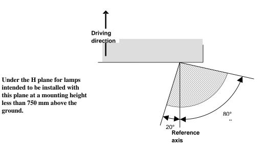
Categories 5 and 6: Supplementary side direction indicators for use on a vehicle also equipped with categories 1, 1a or 1b and 2a or 2b direction indicators
