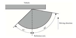
Categories 2a and 2b: Direction indicators for the rear of the vehicle
