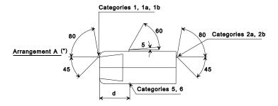
(\*) The value of 5° given for dead angle of visibility to the rear of the side direction-indicator is an upper limit  $d \le 1.80$  m (for  $M_1$  and  $N_1$  category vehicles  $d \le 2.50$  m).
