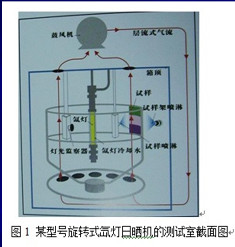
Figure 1 Rotating Drum Xenon Arc Tester Cross Section
