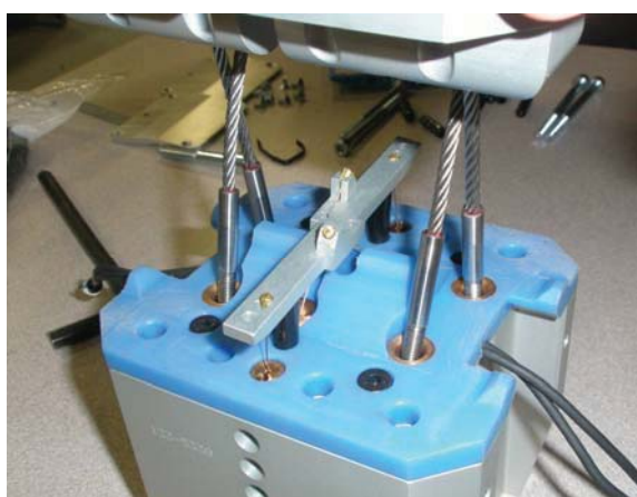
Figure 49 . Cross wire feed through on knee
