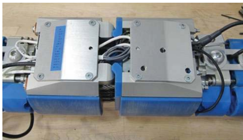
Figure 32 . Left hand side of leg with knee covers fitted. Leg wires are not shown secured
