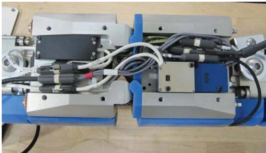
Figure 30 . Typical Slice wiring to knee with SLICE
