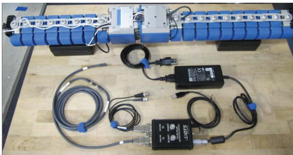
Figure 34 . Leg with disconnect wire, TDAS interface and power supply
