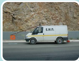
Ground Penetrating Radar (GPR)
