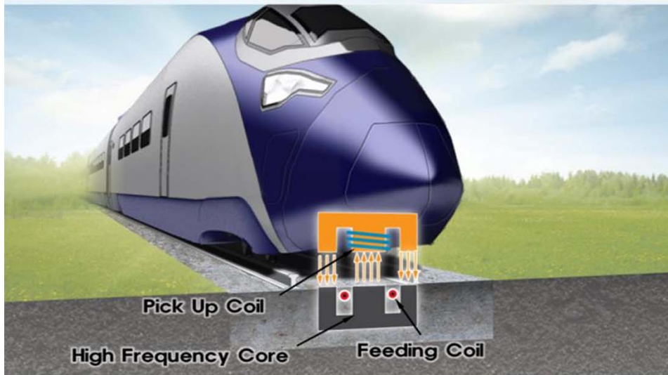
Wireless power transmission enables transmitting high power
