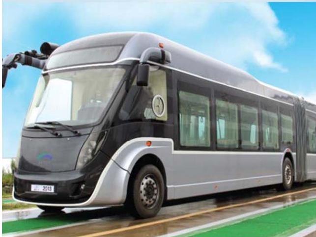
CNG-Hybrid Bimodal Tram Autonomous operation system
