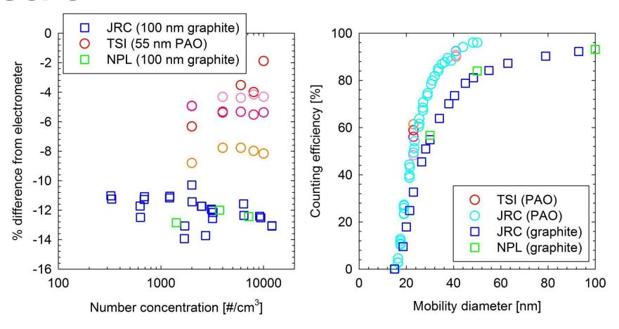
> GCPC exhibits lower detection efficiency for graphite particles even at 100 nm.
