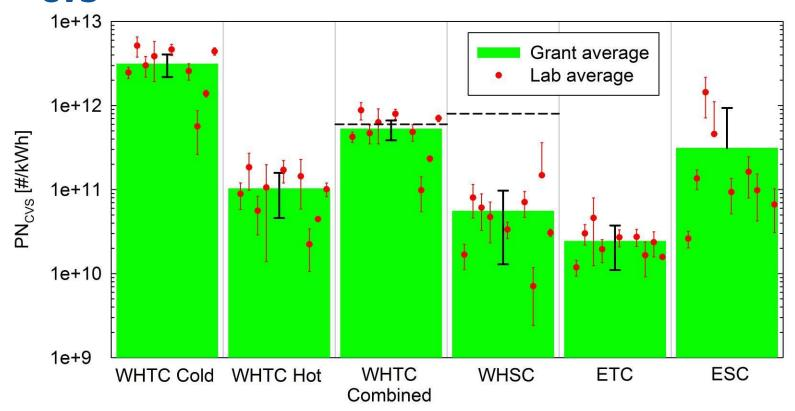
➤ PN emissions complied with the WHSC limit (8×10<sup>11</sup> #/kWh) but were at the threshold value (6×10<sup>11</sup> #/kWh) over the WHTC (14% cold weighting)
