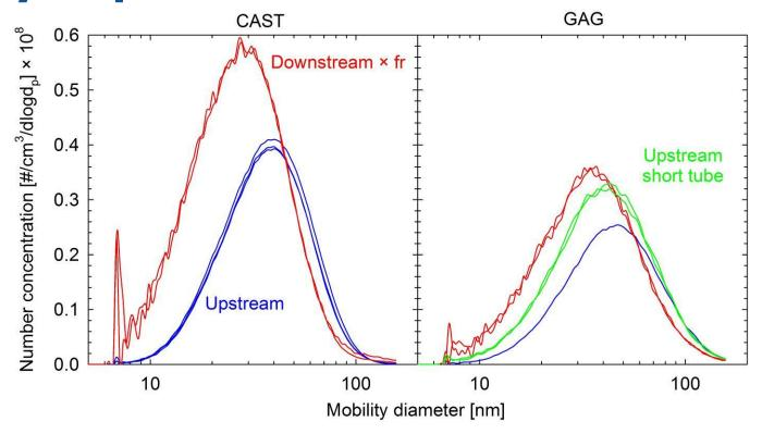
The high number concentrations can lead to significant coagulation. Care needs to be taken to ensure similar residence times when sampling upstream and downstream of the VPR
