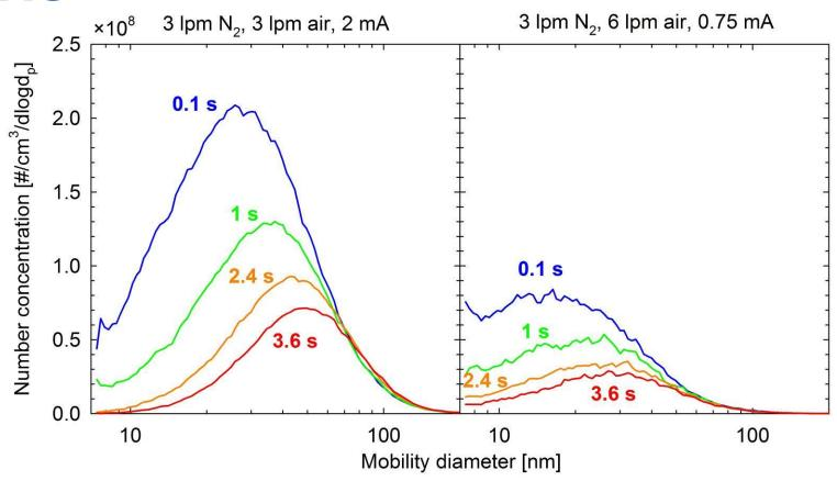
➤ The high number concentration of the aerosol produced by the GAG can lead to significant coagulation, unless immediately diluted.
