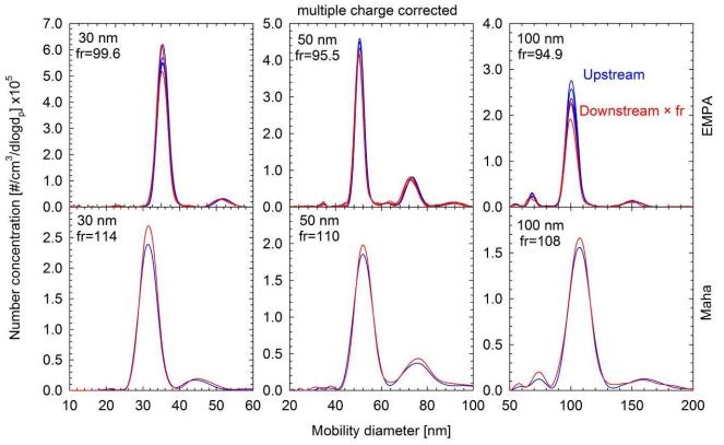
Size distributions of DMA-classified graphite particles upstream and downstream of the GVPR suggest that graphite particles are stable at the 300°C of the GVPR ET.
