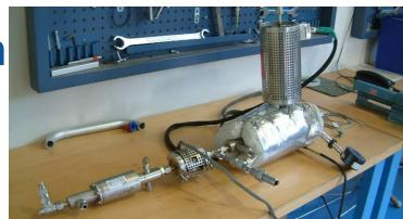
Golden Aerosol Generator (GAG): Palas DNP 3000 graphite spark generator.
