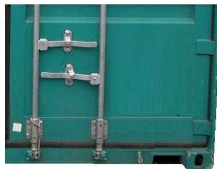
Figure 5.27 Handles between bars
