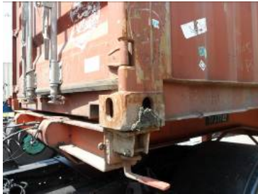
Figure 6.2 Mud in corner fitting
