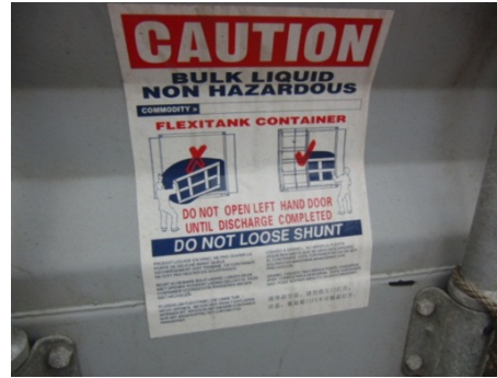
Figure 7.52 Flexitank warning label
