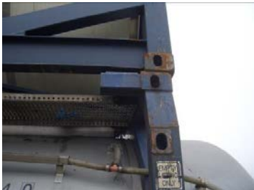
Figure 4.9 Step back with secondary side lift aperture
