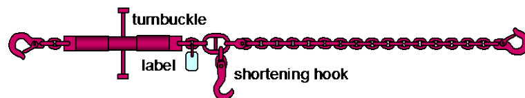
Figure 7.18 Standard chain lashing with shortening hook
