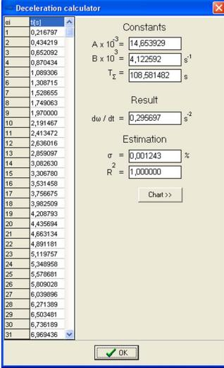
Table 1. Deceleration j at 80 km/h and different speed range. Test machine UTAC1, Tyre 205/55R16, p=0,21 MPa, Lm=482,6daN, R<sub>T</sub>=0,3045 m, I<sub>T</sub>=0,97kgm<sup>2</sup>, Measuring device NAMI-357. Data processing by the "Deceleration Calculator".
