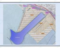
Realization of a reclamation tank, enlargement of the 5th pier, for the dredging mud deposit
