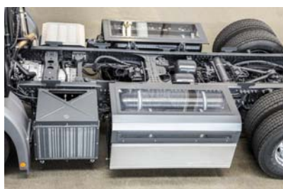
Figure 2: Mercedes Econic 2630 CNG tanks 6
