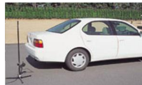
Proximity stationary noise test (No test track is required.)
