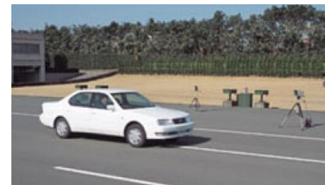
Accelerating/cruising noise tests (A test track is required.)
