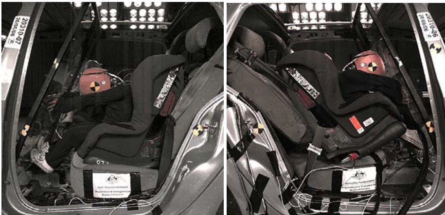
Figure 5 – Frontal impact kinematics for a child restraint model secured to a vehicle using ISOFIX rigid lower connectors and a top tether (left) and a safety belt and top tether (right)
