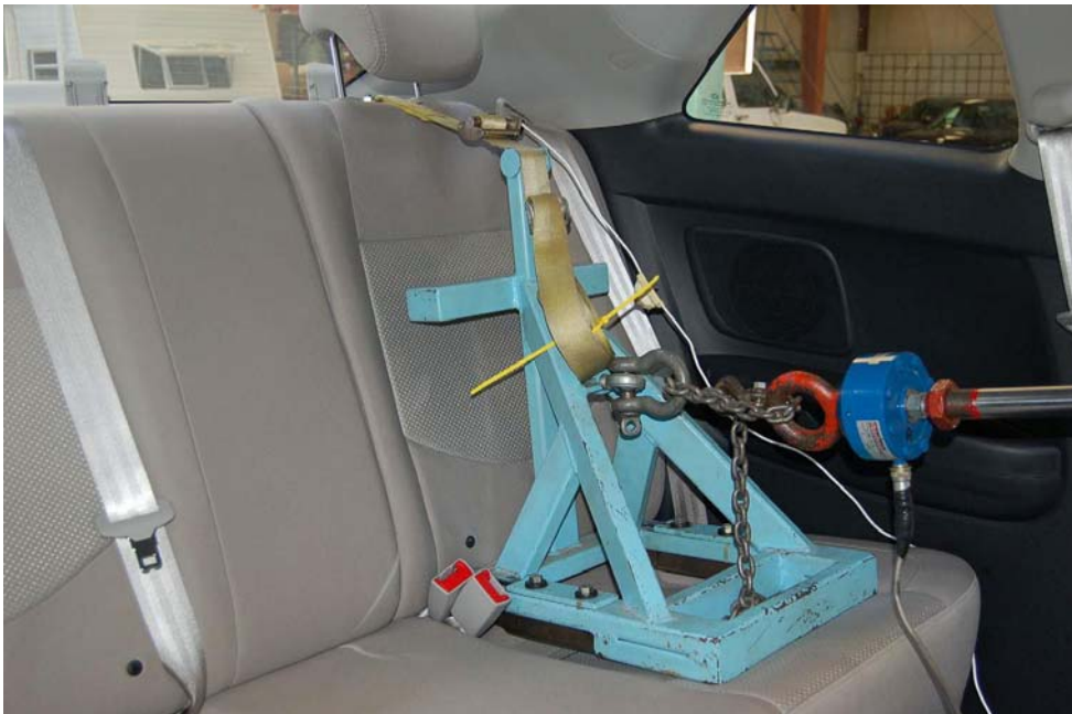
Figure 4 – Example of Static Force Application Device (SFAD) installation (on one side of vehicle only) for an ISOFIX anchorages system and ISOFIX top tether anchorage strength test
