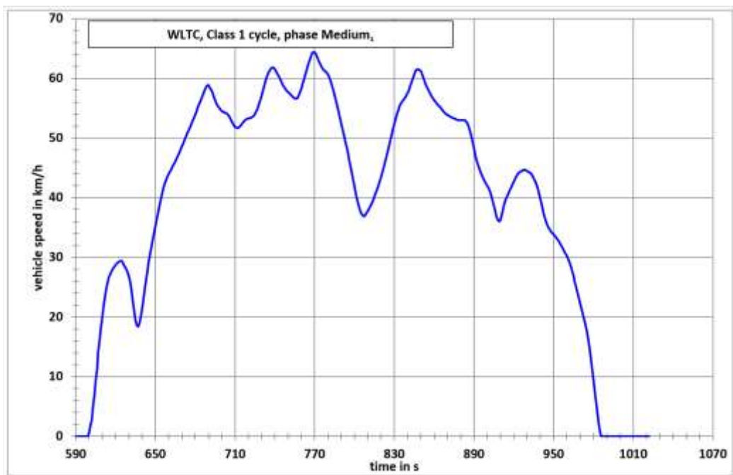
Figure A1/2 WLTC, Class 1 cycle, phase Medium 1
