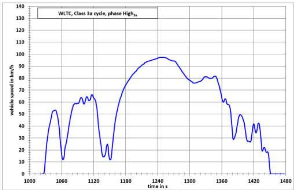
Figure A1/10 WLTC, Class 3a cycle, phase High 3a
