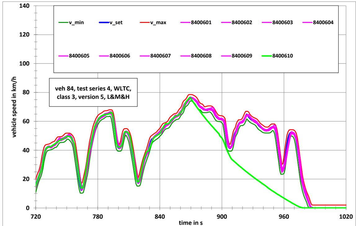
536. The remaining PEV's were all tested on the class 3 cycle.
