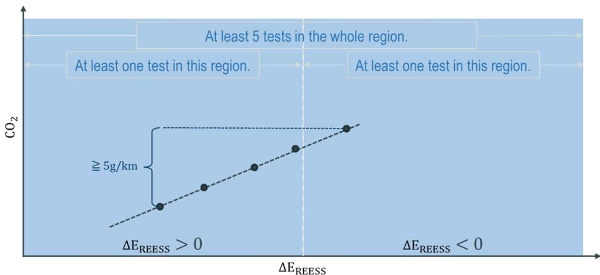
293. In the second step, the required number of tests can be reduced to three tests if the following criteria are fulfilled with respect to the placement of these tests:
