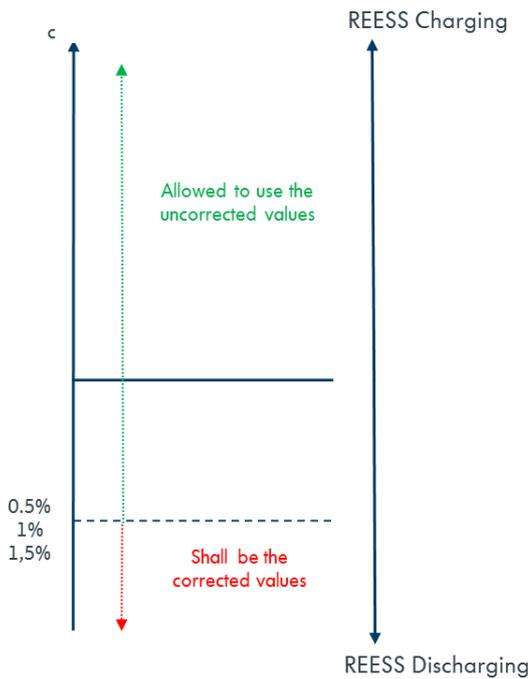
282. Figure 20 is only referring to whole cycle test results. Individual phases have to be corrected irrespective of the energy change, at least if these values are required by the Contracting Party.
