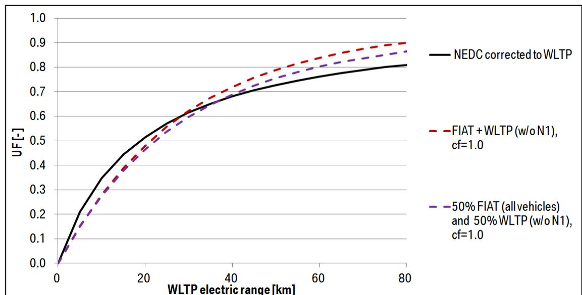
19. In order to compensate for this effect, a 50 % / 50 % weighting approach was applied. For each electric range the respective UF was calculated for both databases and weighted by 50 % for the calculation of the total UF (dashed purple line).
