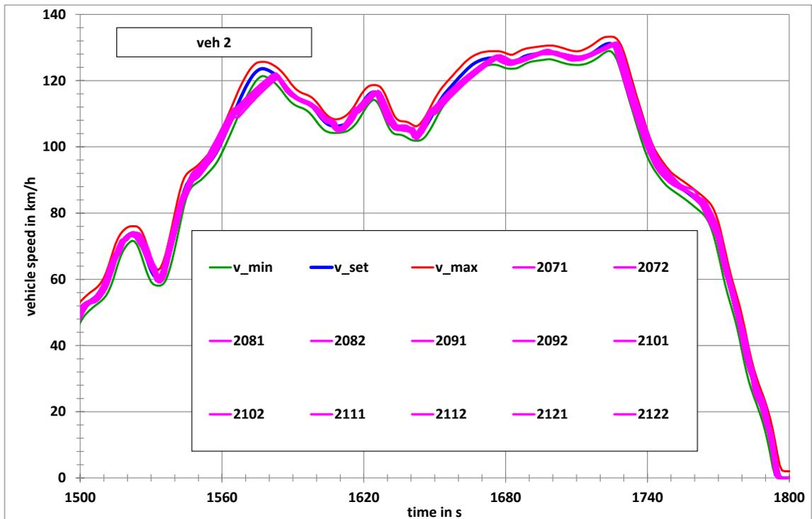
523. A more severe example is shown in Figure 41. This vehicle from India was tested on natural gas, which obviously reduced the maximum power compared to the operation on petrol and would therefore qualify as a class 2 vehicle. In this particular case it would even not be able to reach the top speed of the extra high speed phase of the class 2 cycle (123 km/h).
