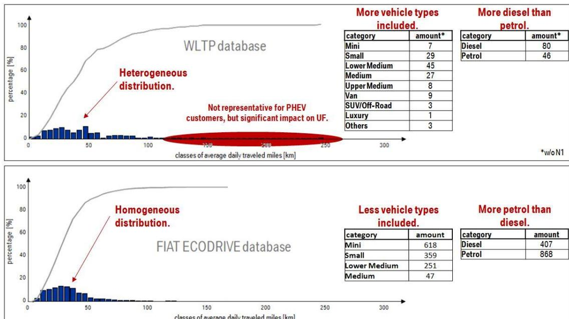
14. A comparison of both databases is shown in Figure 3. The EU WLTP database shows a very wide distribution of driving data and consists of a high share of diesel
