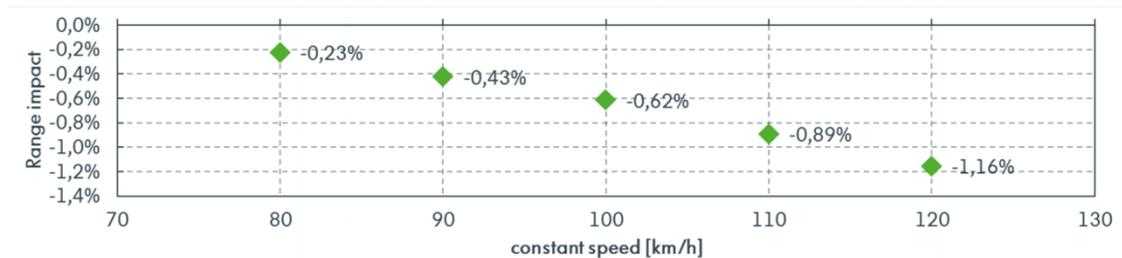
314. Figure 28 shows an additional result provided by JAMA to see the impact of constant speed variations on electric range. The variation width in the range against constant speed was 0.6% between 80 km/h and 120 km/h. The same variation also accounts for the UBE and the energy consumption. Figure 28 only shows results from the shortened test procedure, so there is no comparison to the results for the consecutive test.
