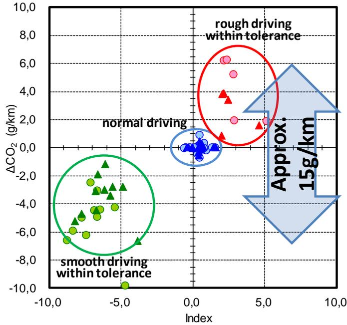
116. This leads to an increase of the test-to-test variation but also to unfair competition. Since the WLTC that was developed is a micro-transient type of test cycle, the current situation may become worse since there is more potential gain in smooth driving.
