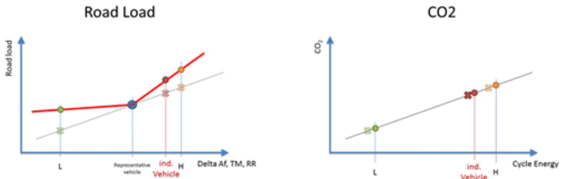
15. The CO<sub>2</sub> measurements for vehicle L and H are performed on a chassis dyno using the road loads of the RLMF calculation. These measured CO<sub>2</sub> values are used for the interpolation of individual CO<sub>2</sub> values based on the individual cycle energy, which is an output of the RLMF calculation. This method is similar to what is already described in the GTR on the CO<sub>2</sub> interpolation for normal passenger cars, and is illustrated in Figure 2.
