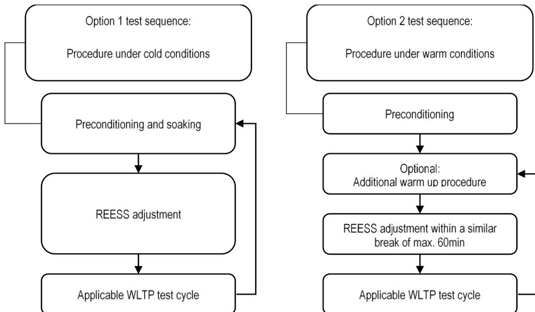
289. Both procedures are repeated until the set of measurement results fulfil the boundary conditions for the correction coefficient determination.
