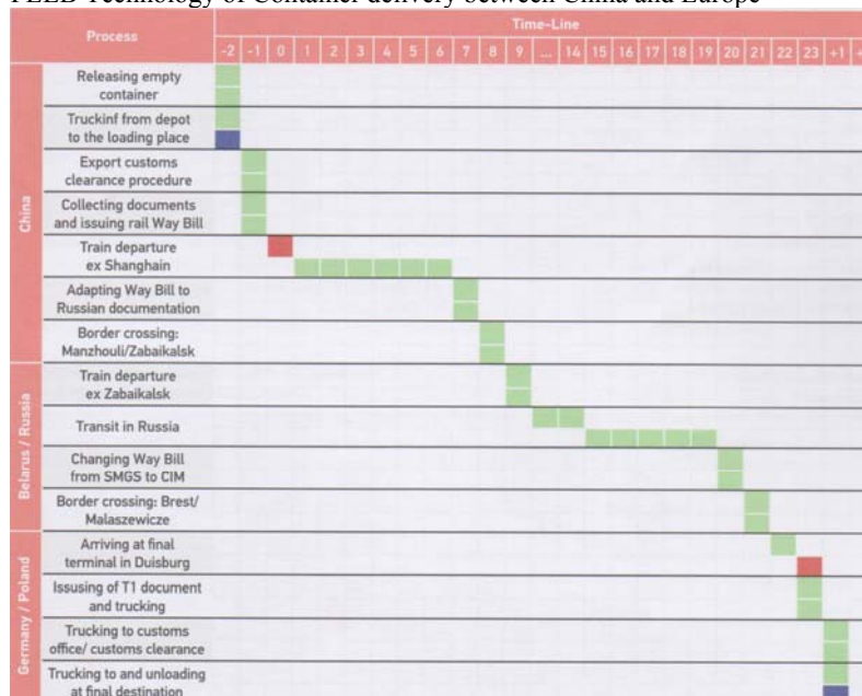
Figure 1.22 FELB Technology of Container delivery between China and Europe
