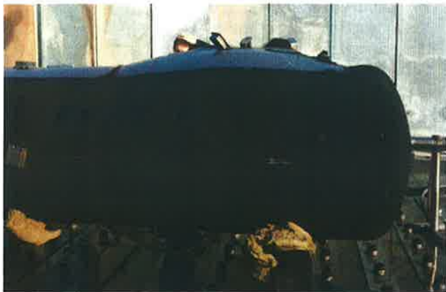
Figure 2. Test 0 - View of deformed and failed B-End
