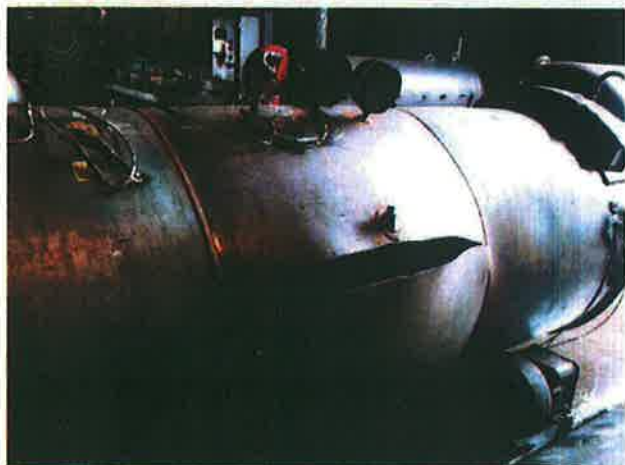
Figure 4. Burst hydrostatic tested tank – Tensile tear
