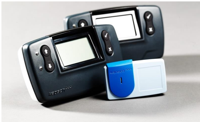
Figure 10: Exemplary figure of a GNSS on-board unit that is mounted on a vehicle's windscreen in comparison to a smaller DSRC on-board unit
