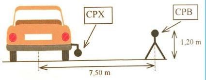
For non-porous pavements and for some porous asphalt pavements, the typical difference between CPX and CPB noise levels in the French data is 22 dB
