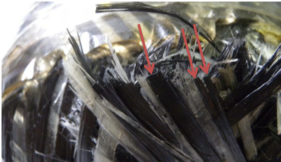
Figure 5-7: Cylinder 5 – Details of sharply truncated fibers after the fatigue test
