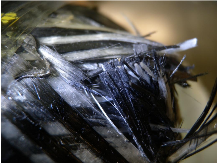
Figure 5-20: Cylinder 11 – Details of sharply truncated fibers after the fatigue test
