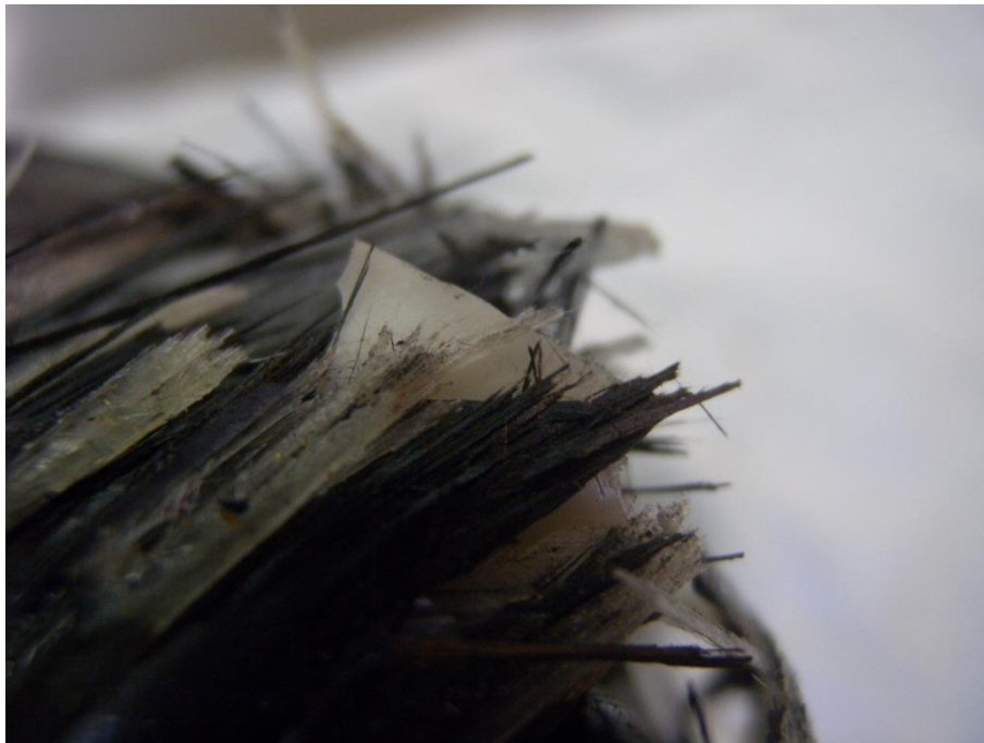
Figure 5-14: Cylinder 7 – Details of sharply truncated fibers after the fatigue test
