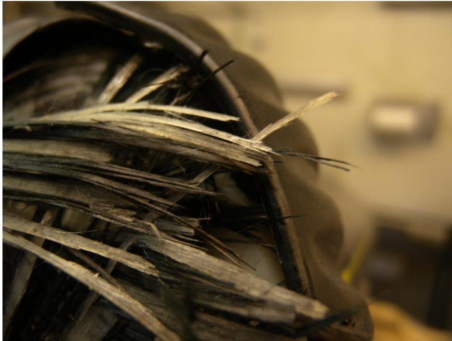
Figure 5-24: Cylinder 12 – Details of frayed fibers after the fatigue test
