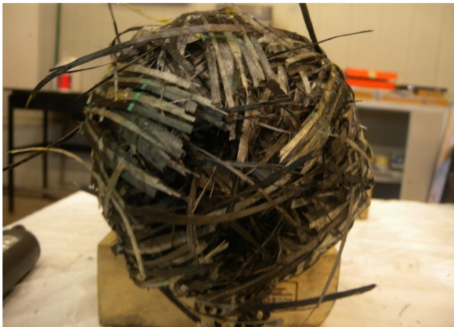
Figure 7-5: Cylinder 10 – Detailed view of the blown up area
