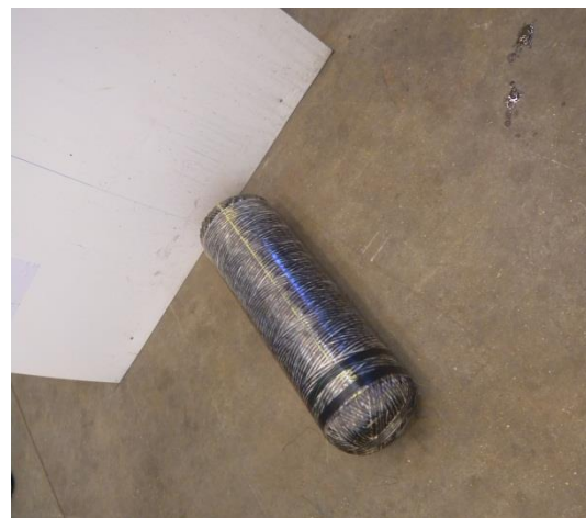
Figure 6-4: Cylinder 2 after the vertical drop, valve side
