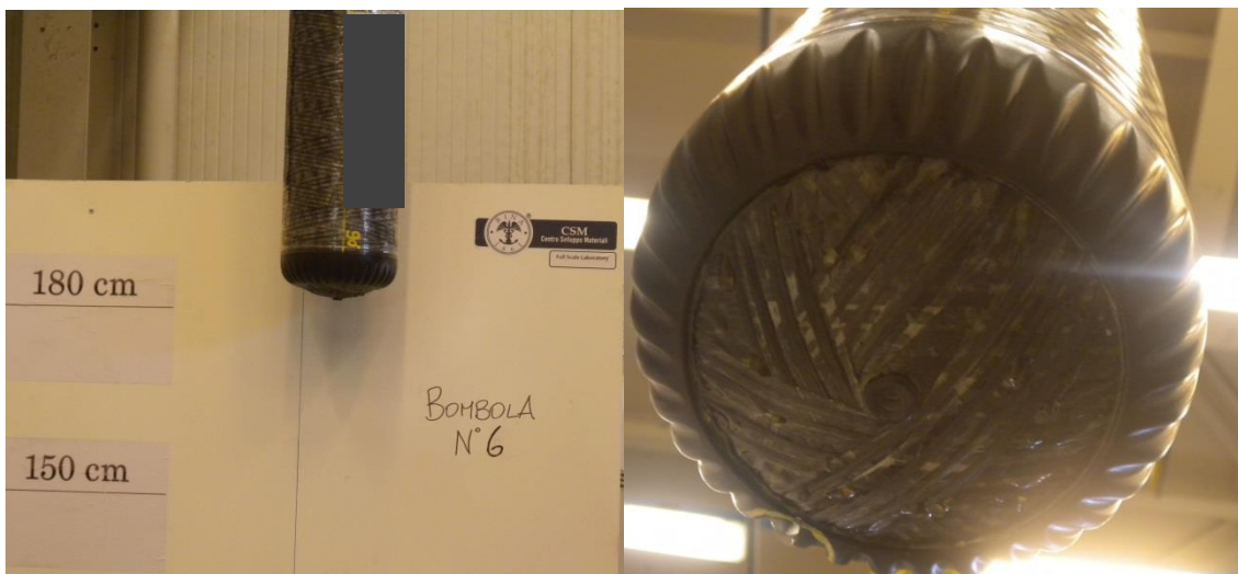
Figure 3-7: Vertical drop on capped side – Cylinder 6
