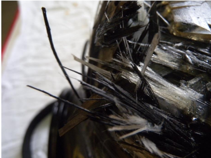
Figure 5-8: Cylinder 5 – Details of frayed fibers after the fatigue test
