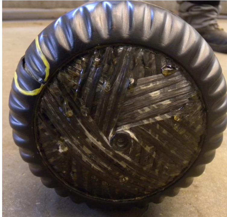
Figure 3-8: Fibers abrasion on the dome after vertical drop, capped side – Cylinder 6
