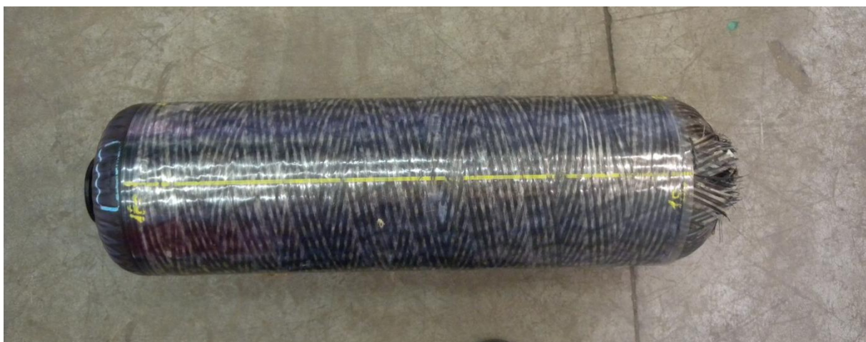
Figure 5-13: Cylinder 7 blown up during the fatigue test
