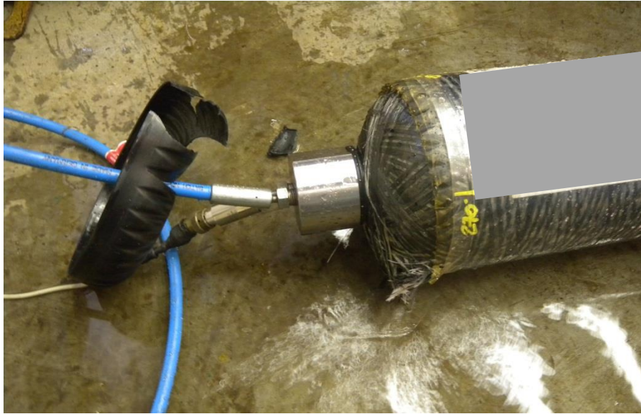
Figure 4-16: Cylinder 3 blown up during the second hydraulic test
