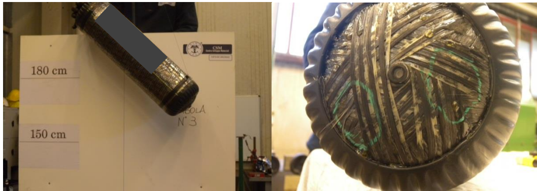
Figure 3-4: Fibers fraying in the dome area after 45° angle drop on capped side – Cylinder 3
