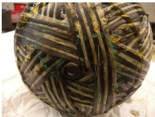
Figure 6-7: Cylinder 10 – Details of damaged fibres after Vertical drop, capped side
