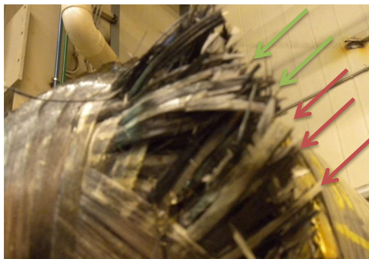
Figure 5-3: Cylinder 1 – Details of broken fibers after the fatigue test
