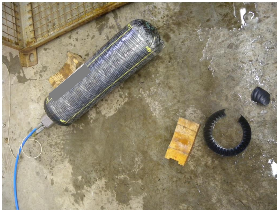
Figure 4-13: Cylinder 3 blown up during the second hydraulic test
