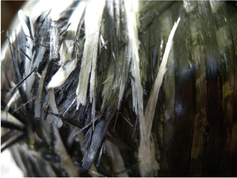
Figure 5-21: Cylinder 11 – Details of frayed fibers after the fatigue test
