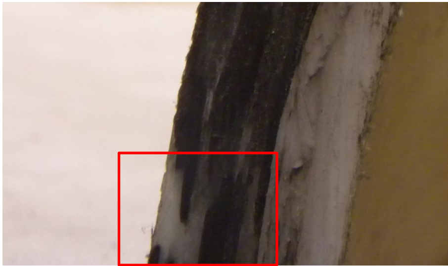
Figure 8-2: Cylinder 7 – Detailed view of the lack of fibers superimposition
