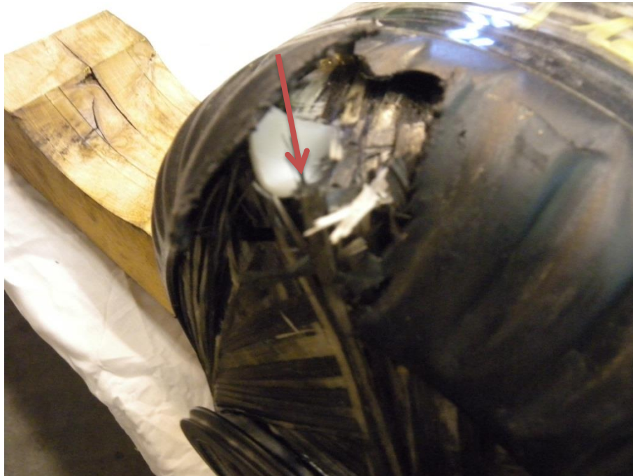
Figure 5-5: Cylinder 4 – Details of broken fibers after the fatigue test
