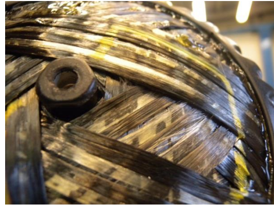
Figure 1-10: Exposed and frayed fibers – Cylinder 5
