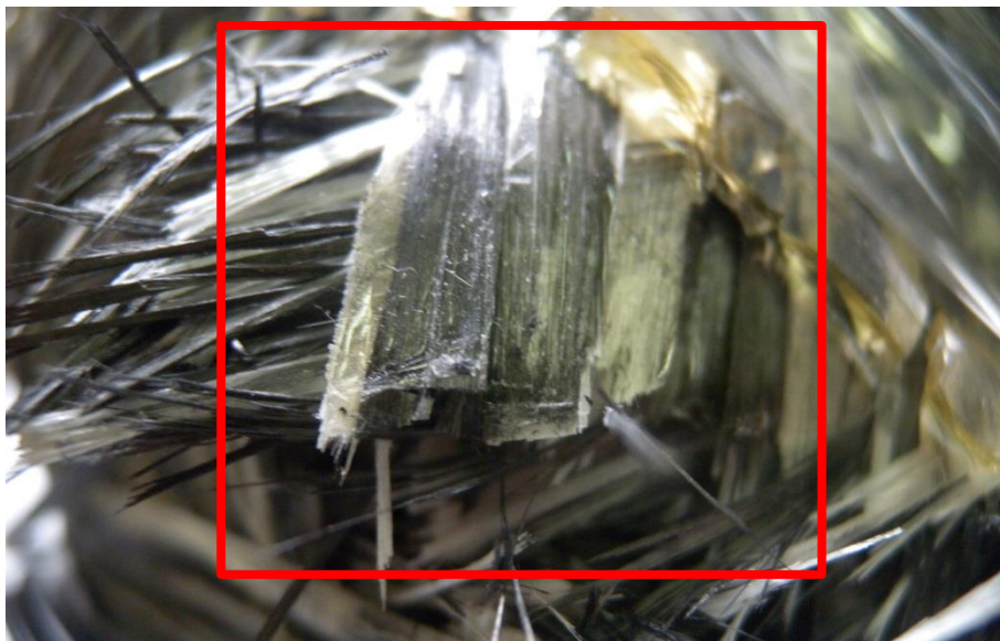
Figure 4-17: Detail of sharply truncated fibers after the second hydraulic test- Cylinder 8
