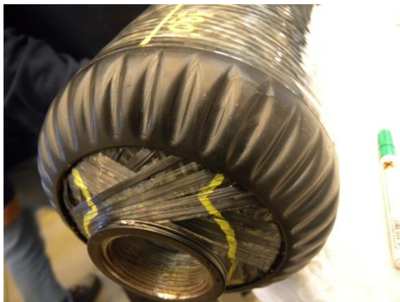
Figure 1-11: Partially exposed fibers – Cylinder 5
