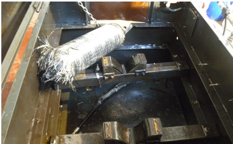
Figure 7-1: Cylinder 2 blown up during the second fatigue test
