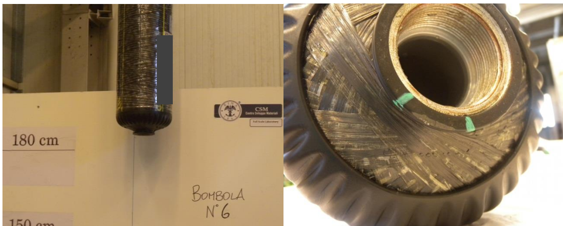
Figure 3-9: Connection abrasion on the valve side after vertical drop – Cylinder 6
