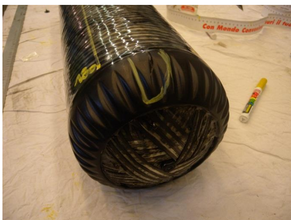
Figure 1-7: Damaged dome – Cylinder 10
