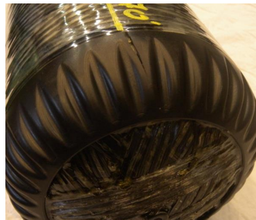
Figure 1-4: Damaged dome – Cylinder 2
