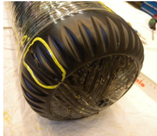
Figure 1-6: Damaged dome – Cylinder 6
