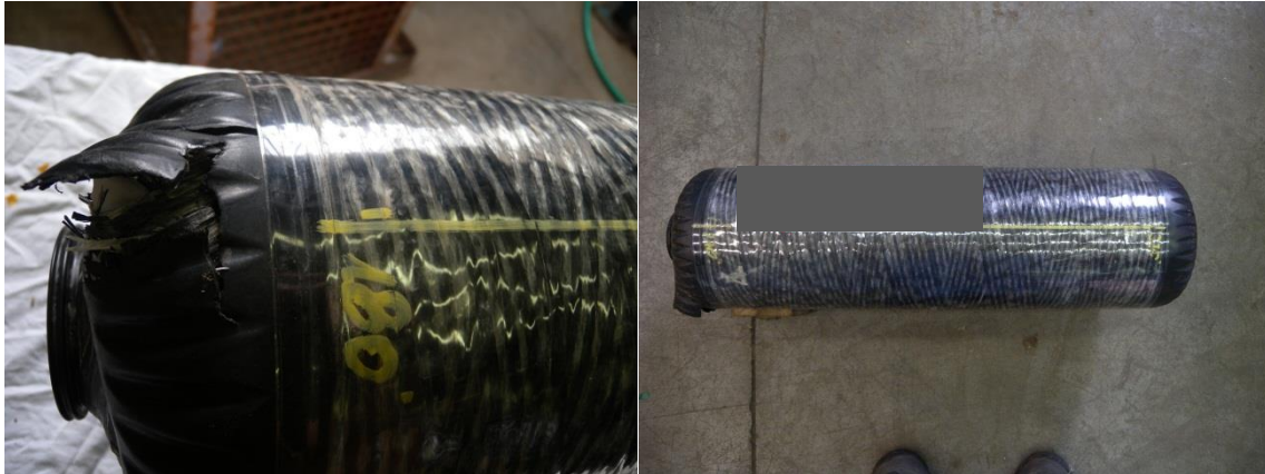
Figure 5-4: Cylinder 4 blown up during the fatigue test
