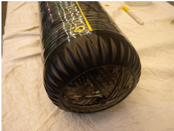
Figure 1-5: Damaged dome – Cylinder 5
