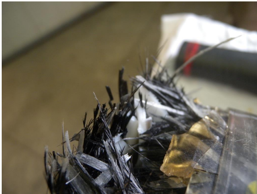
Figure 5-12: Cylinder 6 – Details of frayed fibers after the fatigue test
