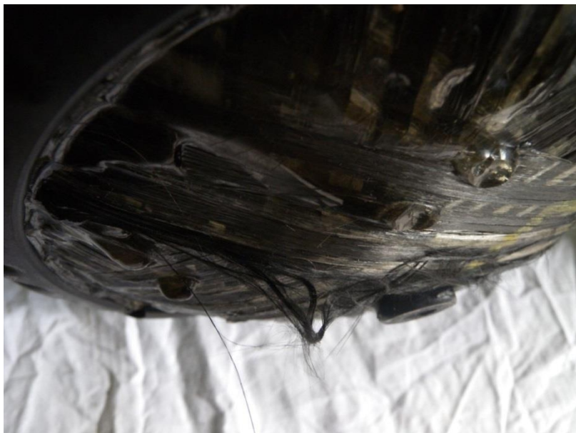
Figure 5-9: Cylinder 5 – Finale state on the fibers after fatigue test in the dome of capped side
