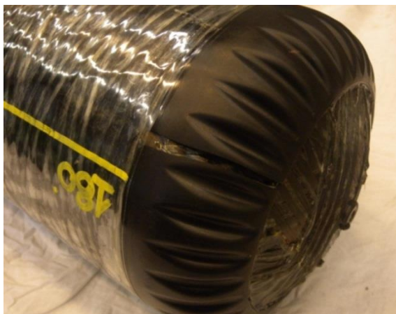
Figure 1-3: Damaged dome – Cylinder 1
