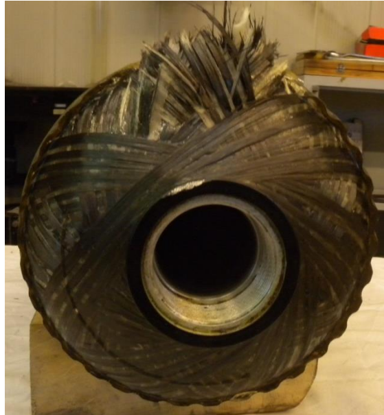
Figure 5-2: Cylinder 1 blown up during the fatigue test
