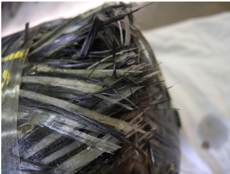
Figure 5-15: Cylinder 7 – Details of frayed fibers after the fatigue test
