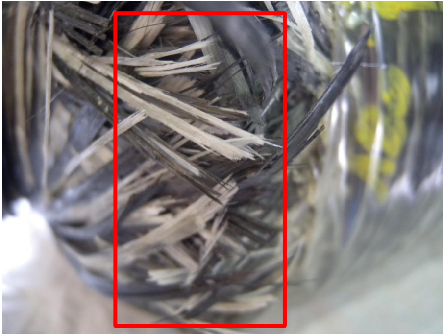
Figure 4-18: Detail of frayed fibers after the second hydraulic test - Cylinder 8
