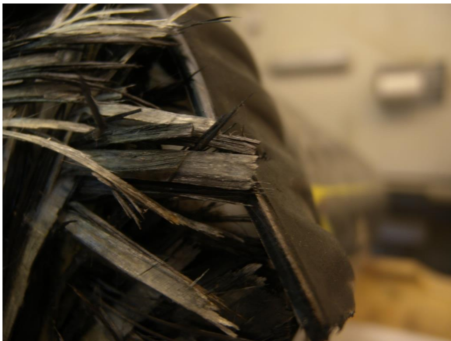
Figure 5-23: Cylinder 12 – Details of sharply truncated fibers after the fatigue test
