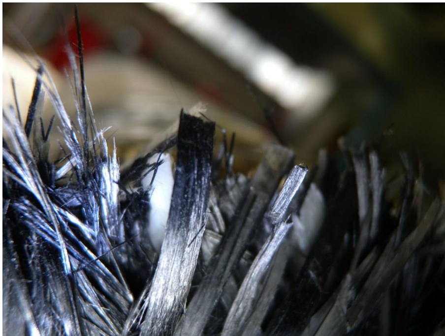
Figure 5-11: Cylinder 6 – Details of sharply truncated fibers after the fatigue test
