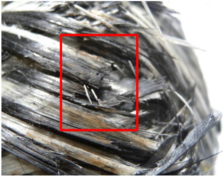
Figure 4-14: Detail of sharply truncated fibers after the second hydraulic test- Cylinder 3
