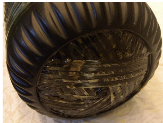
Figure 1-12: Partially exposed fibers – Cylinder 12
