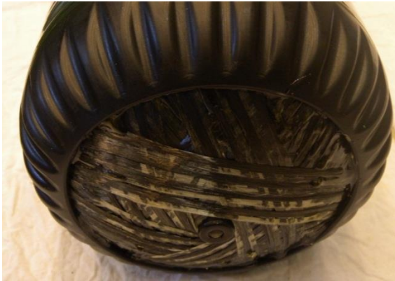
Figure 1-9: Exposed fibers – Cylinder 3
