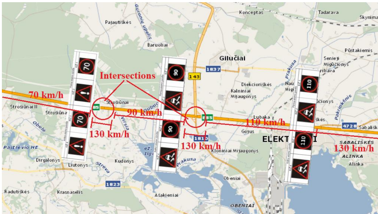
Picture No 1. Road segment of the A1 primary road Vilnius – Kaunas with highlighted intersections and speed limits
