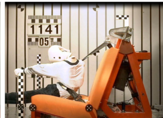
Figure 2c: Time 91 ms – Submarining has already taken place– The lap belt has intruded into the abdomen.
