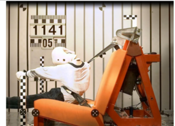
Figure 2c: Time 91 ms – Submerging has already taken place– The lap belt has intruded into the abdomen.
