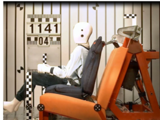
Figure 4b: Time 40 ms – P10 dummy and belt geometry during loading phase
