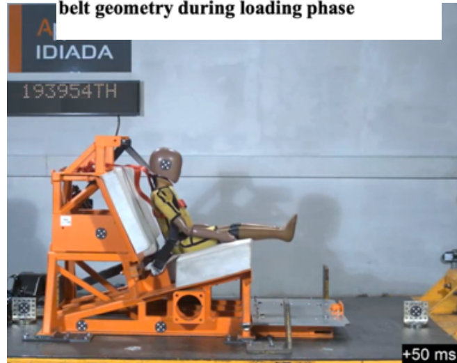
Figure 1b: Time +50 ms – Q6 dummy and belt geometry during loading phase No submerging observed
