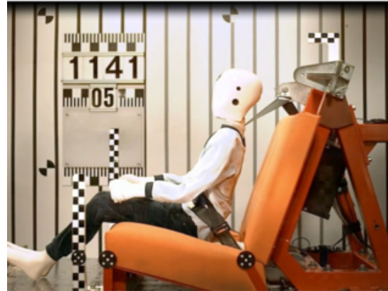
Figure 2b: Time 51 ms – P10 dummy and belt geometry during loading phase
