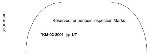
\*Inspection authority mark indicating the month (two figures) and year (four figures) of retest shall be marked at the time when periodic inspection is carried out. Enough space shall be provided, on the cylinder, for more than one reinspection. For acetylene cylinders these stamp marks shall be marked either on the cylinder or on the ring fixed on the top of the cylinder by the valve fitting.
