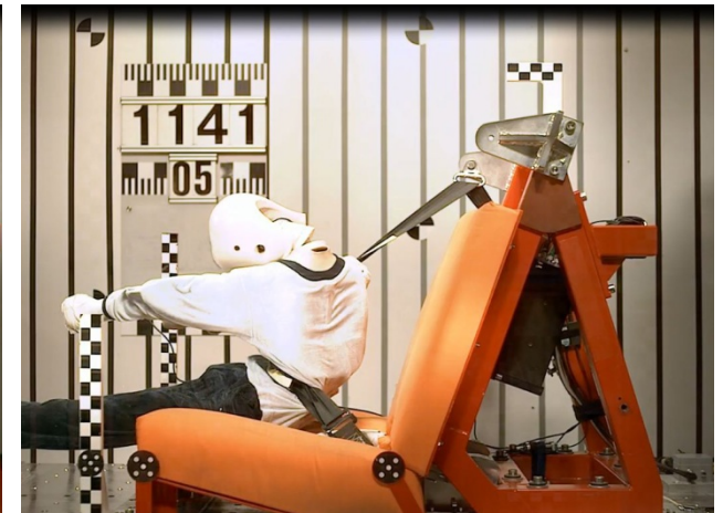
Figure 2c: Time 91 ms – Submarining has already taken place– The lap belt has intruded into the abdomen.
