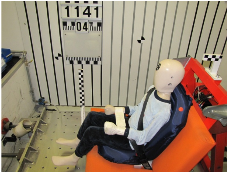
Figure 3: test set-up with the inflatable system
