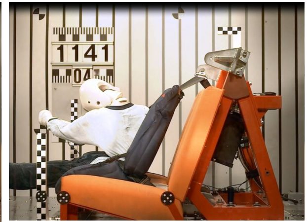
Figure 4c: Time 80 ms – Start of the submarining – The lap belt has intruded into the abdomen.
