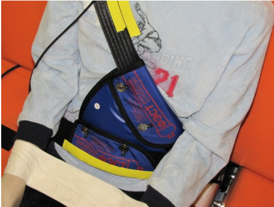
Figure 1: test set-up with belt guide device using the P10 dummy
