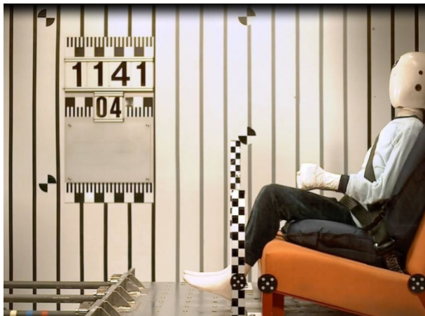
Figure 4a: Time 0 ms – Initial P10 dummy position
