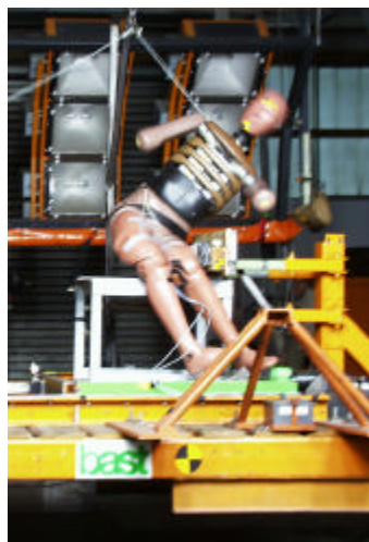
Figure 15: ES-2 prototype and EUROSID-1 in sled tests at BAST, impact speed 20 km/h; impact direction 20 degrees aft (pelvis contact first), Left: EUROSID-1 (equipped with US-SID legs) during impact.
